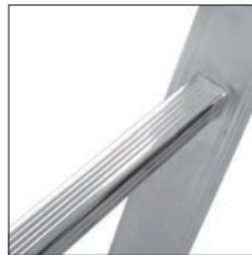
Square-section (25x25 mm), knurled, slip-proof rungs.
