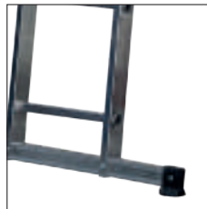
Compulsory stabilizer bar to use according to EN131 standards. Width: 900 mm with 14 and 16 rungs, 1200 mm with 18 rungs. Removable for transportation purposes.
